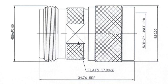
MATERIAL : BODY-BRASS CONTACT-BRASS INSULATOR-PTFE SHELL-BRASS C WASHER-BRASS GASKET-SILICONE SLEEVE-BRASS FINISH : BODY-TRI-ALLOY PLATING CONTACT-GOLD PLATING OVER NICKEL SHELL-TRI-ALLOY PLATING SLEEVE-TRI-ALLOY PLATING
